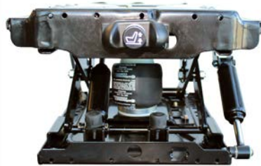
Double Damper View
