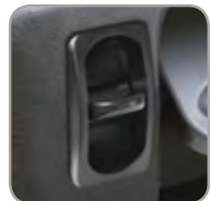
COMPRESSOR SWITCH/AIR RELEASE VALVE
