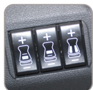
ADJUSTABLE AIR LUMBAR & AIR BOLSTERS
