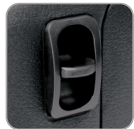
COMPRESSOR SWITCH/AIR RELEASE VALVE
