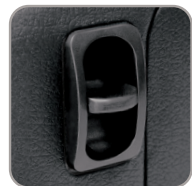
COMPRESSOR SWITCH/AIR RELEASE VALVE
