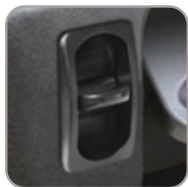
COMPRESSOR SWITCH/AIR RELEASE VALVE
