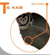
Locate the weld nut as indicated in the illustration
