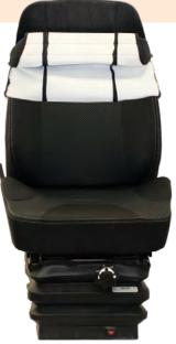
Pull lower portion of the back cover downaround the seat cushion ensuring the elastic is fully under the seat cushion and not sitting on the edge.
