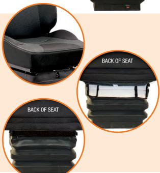
On the front portion of the back cover push the velcro strip through the gap between back of the seat and seat cushion. Pull tight and secure velcro edges together.
