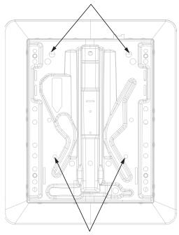
REQUIRES REMOVAL OF 2X SOCKET CAP BOLTS FOR ACCESS TO WELD NUTS.REQUIRES 4X 200264 WASHERS (ADDITIONAL 1X200280 FOR LESS THAN 12")FOR CLEARANCE TO MOUNT FLUSH FOR EACH SIDE .
