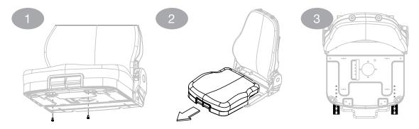
NOTE: TEMPORARILY REMOVE SEAT CUSHION TO ACCESS FRONT HOLES IN SLIDE RAILS.
