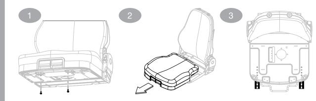
TEMPORARILY REMOVE SEAT CUSHION TO ACCESS FRONT HOLES IN SLIDE RAILS
