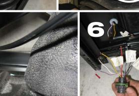
Feed the wires through the plastic plug in the bottom of the suspension.
