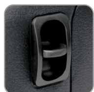
COMPRESSOR SWITCH/AIR RELEASE VALVE
