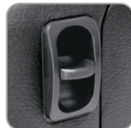
COMPRESSOR SWITCH/AIR RELEASE VALVE
