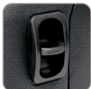
COMPRESSOR SWITCH/AIR RELEASE VALVE
